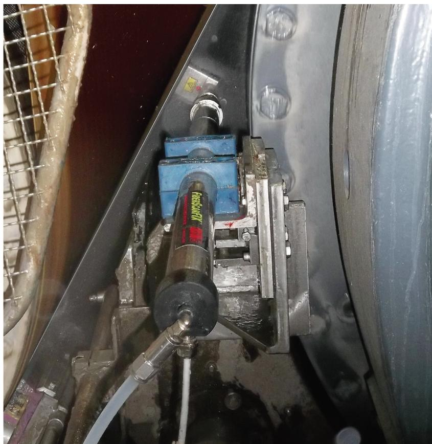
**Figure 1.** FiberScanFIX microwave sensor installation point in restricted areas
