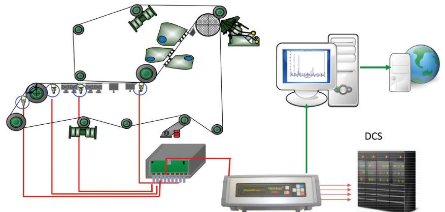
Figure 3. FiberScanFix system layout
