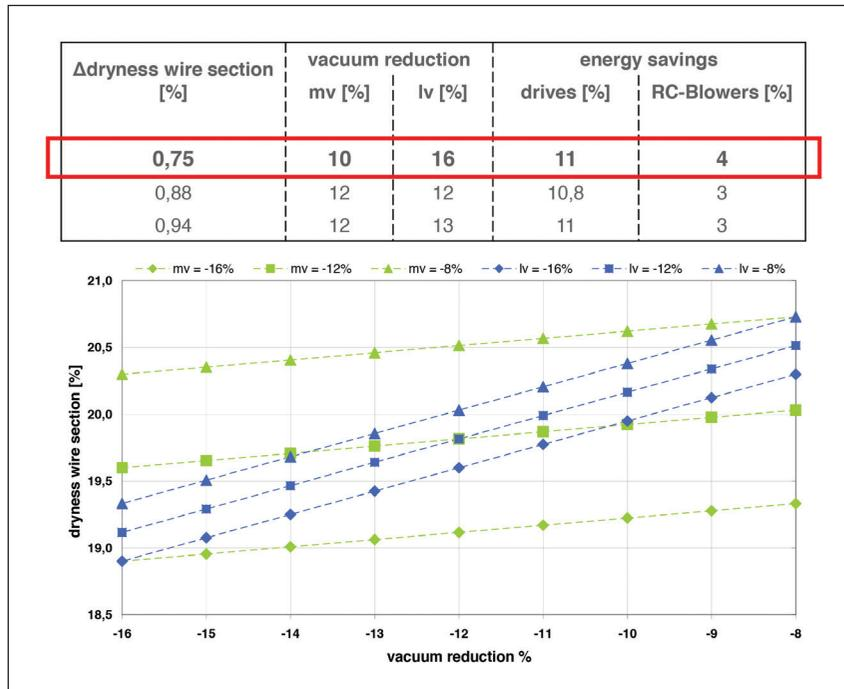
Figure 5. Vacuum reduction vs energy saving
